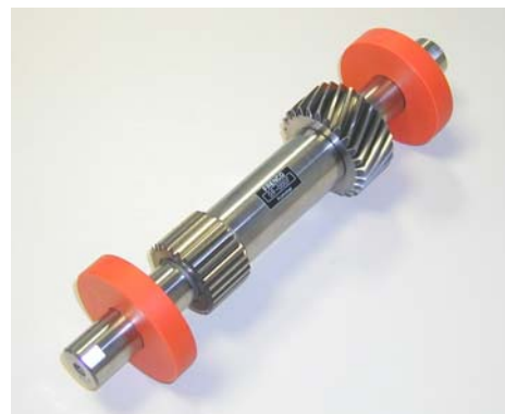
Artefact for the calibration of URM measuring instrument
