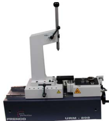
Single end mounting for the workpiece. Left side: steady center attachment to mount the master gear (accessory)
