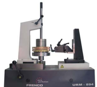
Measurement of worm gears with an according adaptor (accessory)
