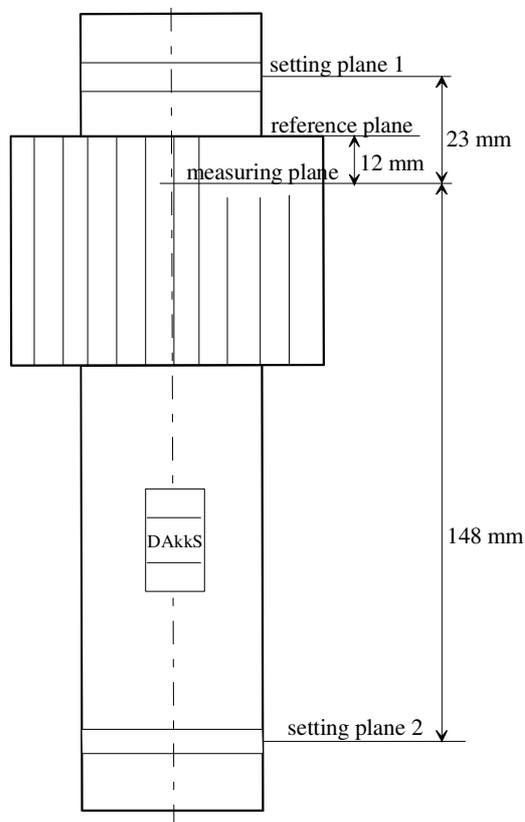
Figure 1: Position of the reference plane and the measuring plan
