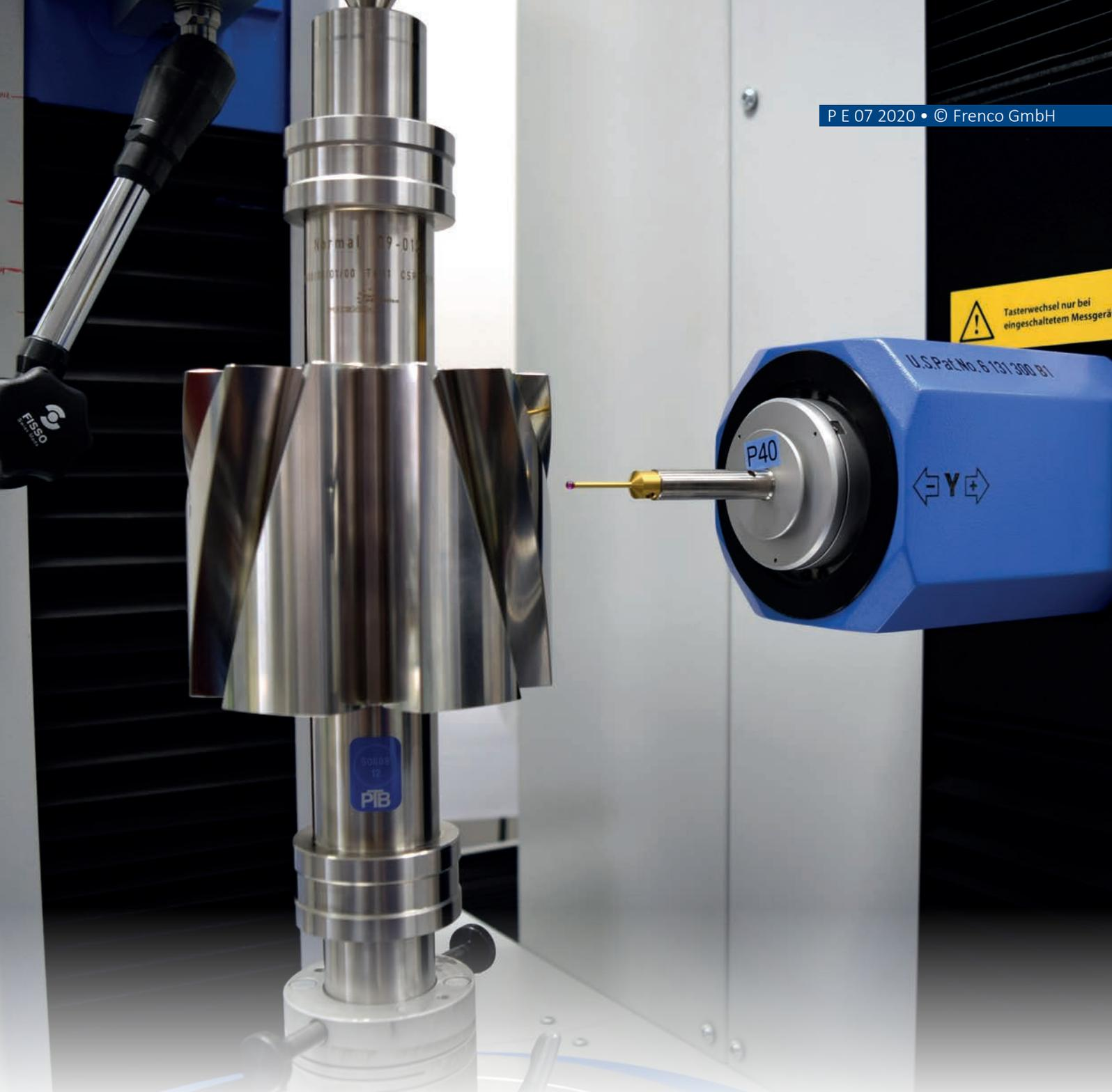
**Gear and Spline Inspection according to certified standards**
