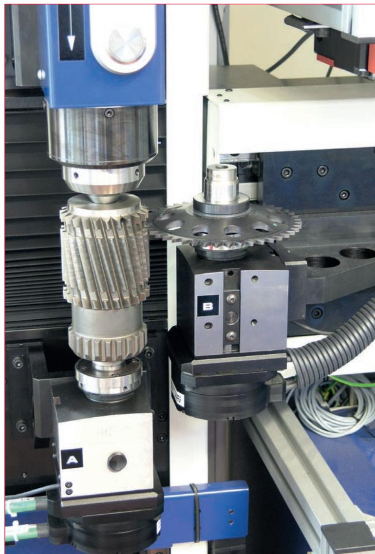
Depending on the number of teeth and the device, the entire gear profile can be scanned within 3 to 13 minutes. It is possible to evaluate a large number of other parameters, besides the usual parameters, such as profile, pitch and runout, with the measuring time remaining the same.
