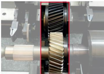
Double flank gear roll test
