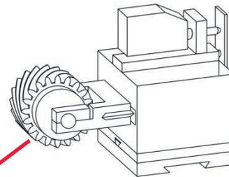
Measuring slide with master gear for a double flank roll test
