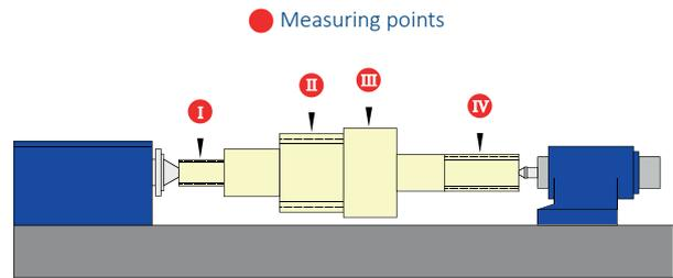
The axes of the individual geometrical elements of the workpiece can be determined and offset against each other.
