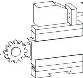
Measuring slide with measuring wheel for splines
