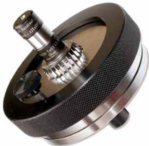
Franco concentricity ring for runout checking.
