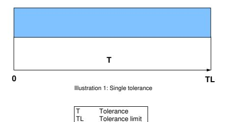
If a specimen is supposed to be accepted as correct the actual value of a feature should not exceed the tolerance limit. The actual value, however, is only a theoretical one. In practice there is only a measured value which was determined with a certain measuring uncertainty.
