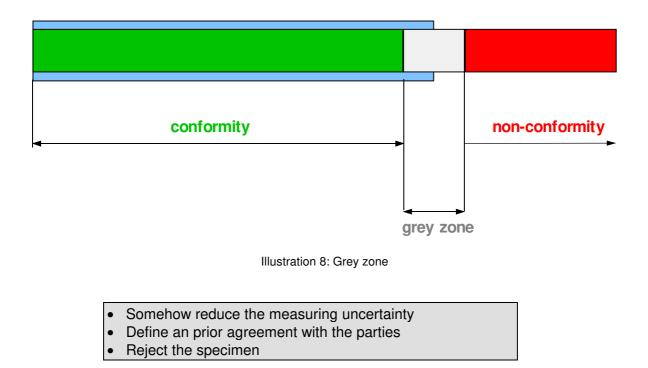
Before starting the measurement, the practical handling of specimen with a measured value within the grey zone should have been clarified. The ISO 14253 indicates that, if no arrangements have been made, work pieces with a measured value within the grey zone should be rejected. Therefore, the following two specimen would be rejected:
