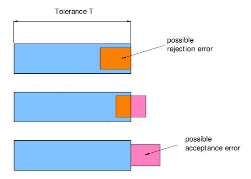
Illustration 18: Scaled representation of tolerance and error
