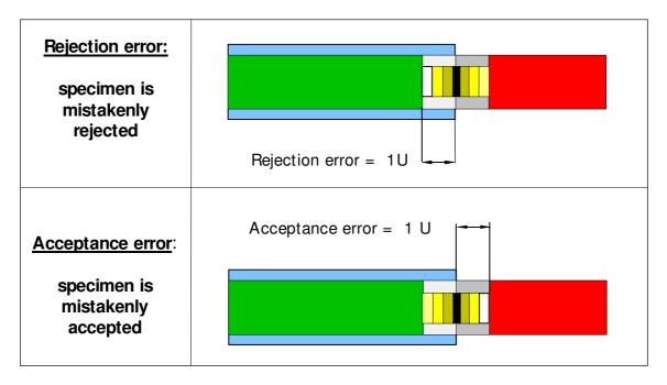
Agreement A can create both a rejection error and an acceptance error:
