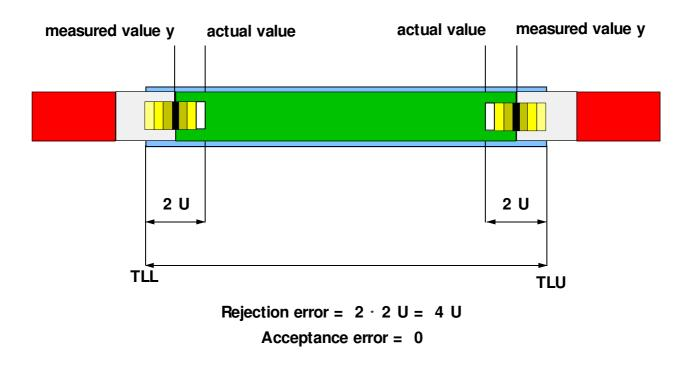
Illustration 12: Rejection error with bilateral tolerance limits
