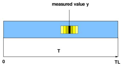
Illustration 3: Measured value y within tolerance
