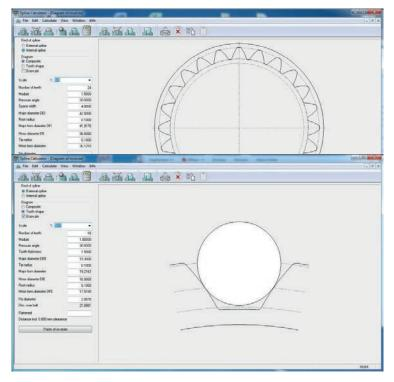
For CAD systems, up to 100 involute points can be calculated for a flank and saved as a text file. This makes it easier to draw up gearing profiles in CAD.
