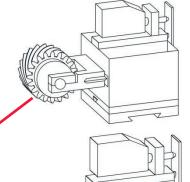
Measuring slide with master gear for a double flank roll test
