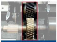
Double flank gear roll test
