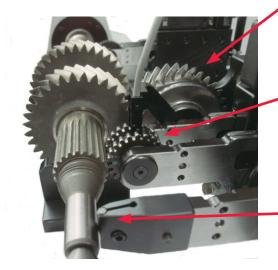
Measuring slide with measuring wheel for splines
