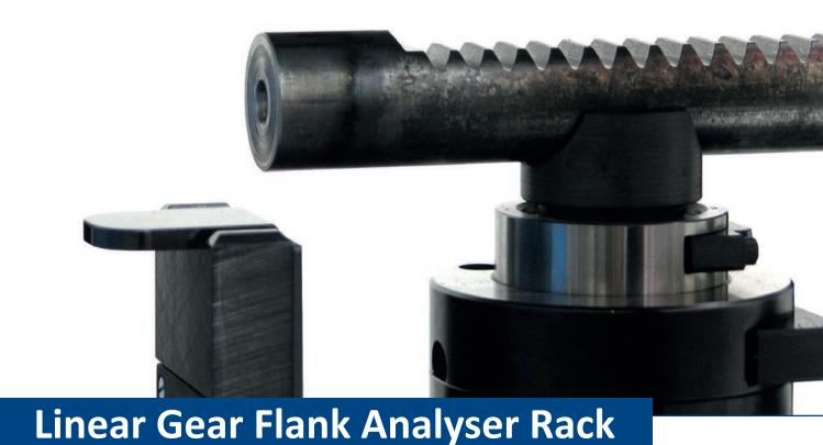
Quality control based on double flank gear roll inspection
